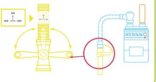
If you smell gas, after following these steps turn the emergency control valve off again and call the National Gas Emergency Service for free immediately on 0800 111 999. This line is in operation 24 hours a day. To stay safe, it's important that you do not try to turn any appliances back on. Keep your windows and doors open until an engineer arrives.
